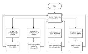
Figure 9: Flow Diagram
