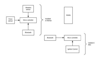
Figure 1: Block Diagram
