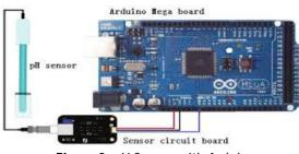
Figure 2: pH Sensor with Arduino
