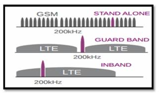
Figure 2: NB-IoT Deployment option [8]
